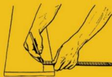
Measure to find the centre of the room, and snap two chalk lines that intersect exactly in the centre of the floor.
