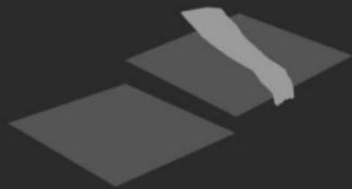
An advantage you have with tiling a floor over tiling a wall is you can dry lay a few rows of tiles first and therefore make necessary cuts and adjustments to tiles beforehand.
